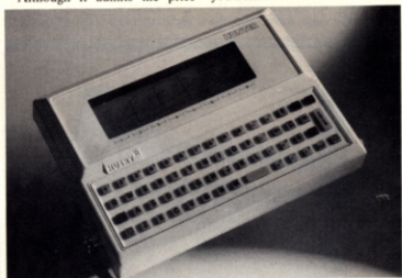
Husky's Hunter — a tough portable with 70K of non-volatile memory.
